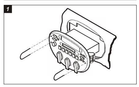
Disconnect the negative battery terminal to prevent an accidental short circuit. Reach under the driver's side dash and unclip the temperature control cable. Using Metra's 86-5618, pull the factory radio/climate control panel from the dash. Disconnect the switch power harness, antenna plug, radio/speaker power harnesses and vacuum hose harness.
